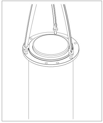
13 - After positioning the bollard inside the case, remove the lifting eye-bolts and, using the same holes, position the blocks on the pipe guide ring.
