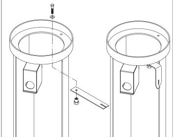
5 -Fit the clamps as in the figure locking them in position with the washer and the M10 hexagonal head screw. Fold them according to the foundation.
