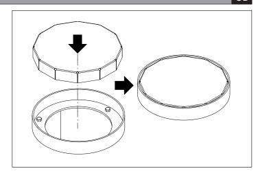
8 - Before inserting the bollard into its housing, remove the previously placed closing or cover making sure that the anchorage housing of the bollard, represented by the grey area, is cleaned carefully. See figures alongside.
