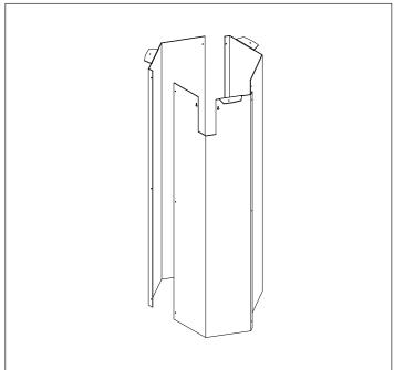
2 - Using the round head screws provided, assemble the hexagonal structure. It is very important to assemble the three elements vertically and on a surface that ensures excellent flatness so as to obtain a reliable support surface for the closing flange. Attention: The screw head must be placed on the internal side of the foundation case. See figure alongside.
