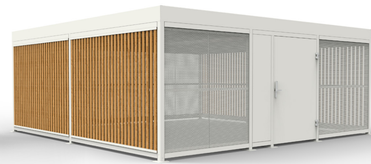
6m frontage x 6m depth Perforated metal sheet frontage and backside Wooden battens cladding on the sides
