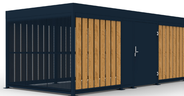
6m frontage x 3m depth Wooden planks cladding frontage and backside Perforated metal sheet on the sides
