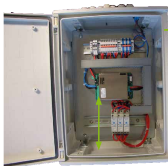
management and production box incorporating an ENDURANCE + 690Wh lithium battery
