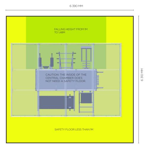
8 HOURS WITH 4 PEOPLE + A CRANE OR A FORKLIFT CONCRETE MEMBER SURFACE SQ.M 40,25 SQ.M FALLING HEIGHT FROM 1M SQ.M TO 1,48M 10,50 SQ.M SAFETY FLOOR LESS THAN 1M **26,50 SQ.M** SQ.M PERIMETER Im 25,40 LM
