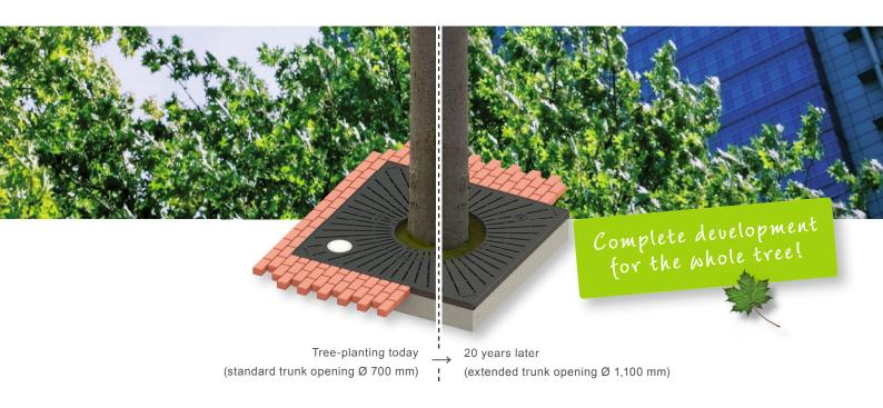
Grows with the task: The internal diameter can be extended from 700 mm to 1,100 mm by simple grinding off at the intended cutting points (except 1,250 x 1,250 mm und  $\varnothing$  1,500 mm).
